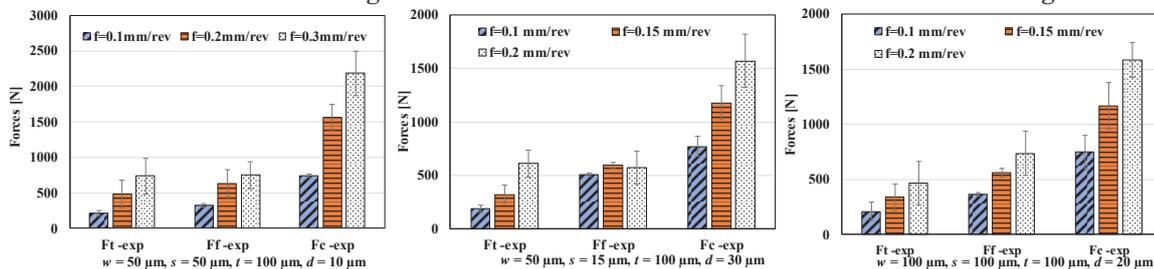
**Fig. 3:** Measured cutting forces using micro-grooved tool for varying feed rate, ( $v_c = 90 \text{ m/min}$ ,  $a_p = 2 \text{ mm}$ ).
