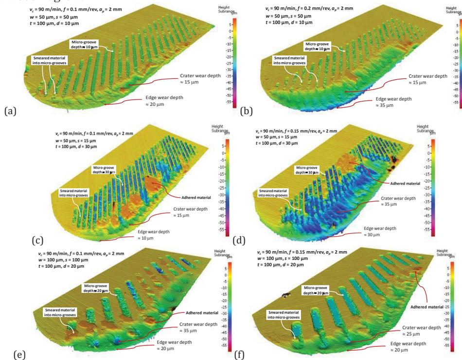
**Fig. 4.** The areal height maps obtained from micro-grooved tool rake faces.
