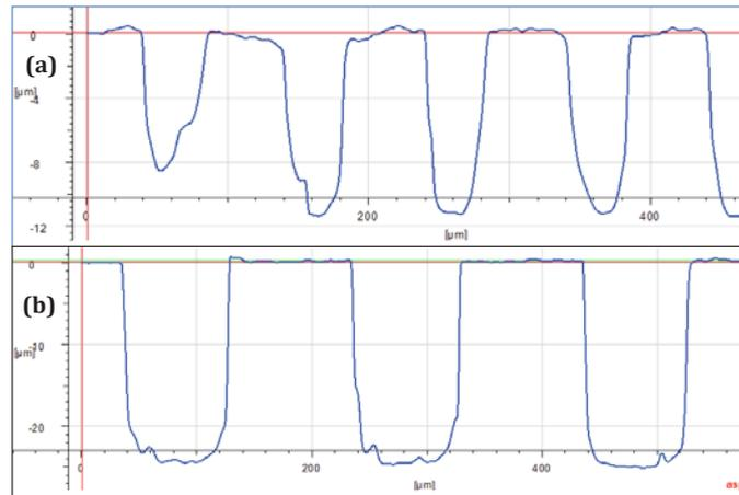
**Fig. 2.** Profile measurement of micro-grooves on the tool surface with micro-grooved pattern parameters; (a)  $w = 50 \mu\text{m}$ ,  $s = 50 \mu\text{m}$ ,  $d = 10 \mu\text{m}$ , and (b)  $w = 100 \mu\text{m}$ ,  $s = 100 \mu\text{m}$ ,  $d = 20 \mu\text{m}$ .
