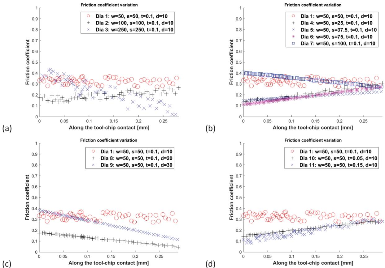
Fig. 9: Effects of micro-grooved tool design parameters on variable friction coefficient.
