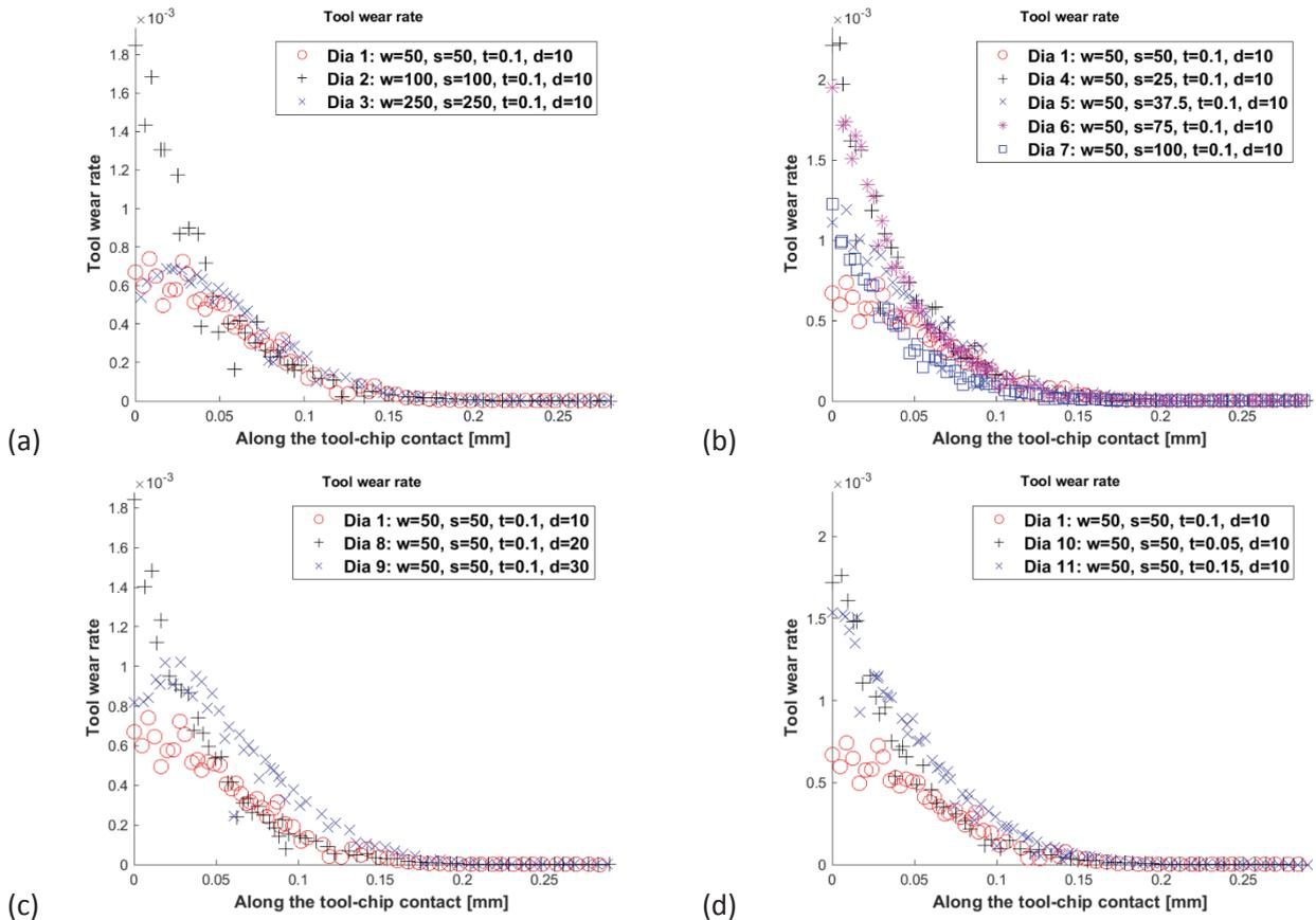
Fig. 8: Effects of micro-groove parameters on tool wear rate.
