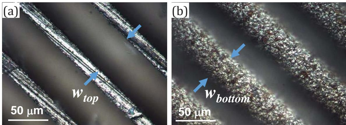
Fig. 1: Images of micro-grooves at the top (a) and the bottom (b) surfaces (micro-groove parameters;  $w = 50 \mu\text{m}$ ,  $s = 15 \mu\text{m}$ ,  $t = 100 \mu\text{m}$ ,  $d = 30 \mu\text{m}$ ).
