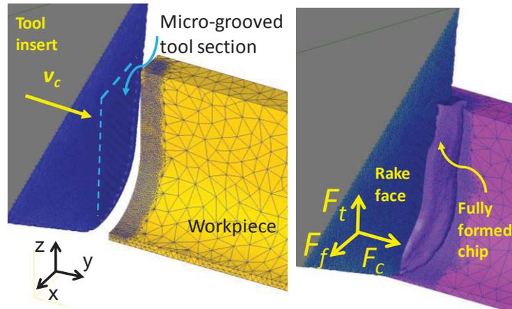
**Fig. 5:** Finite element model of turning using micro-grooved tool.
