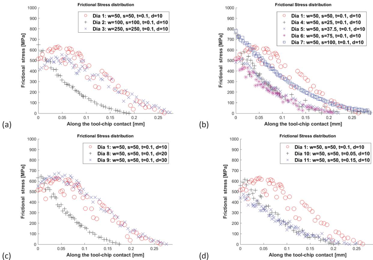
Fig. 6: Effects of micro-groove parameters on the frictional stress along tool-chip contact.
