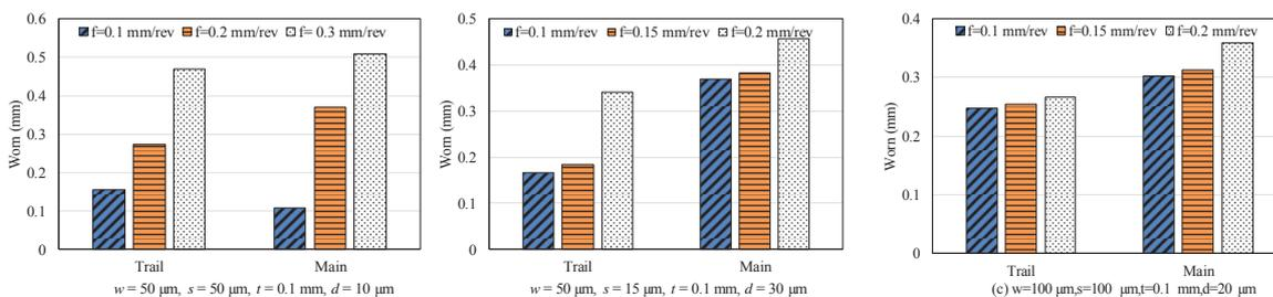
Fig. 7: Tool rake face wear against the feed rate.
